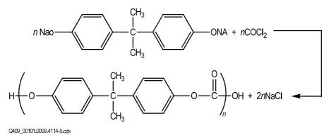
Polycarbonate can also be produced via solution or melt processes, but only the melt transesterification process has found commercial viability in recent years, largely due to its environmental superiority.
