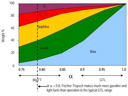
F-T Designed to Maximize Gasoline Production
