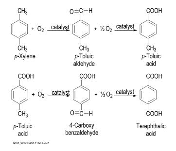
Purification of CTA requires at least one chemical step in addition to the physical procedures (e.g. crystallization, washing). One of the major impurities, 4-carboxybenzaldehyde (4-CBA), is quite difficult to remove by physical means but can be converted to *para*-toluic acid by catalytic hydrogenation in an aqueous solution, as shown in the following equation:
