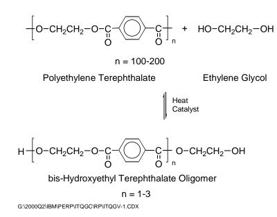
In the Eastman process, ethylene glycol is added to the polyester at a mole ratio of glycol to dicarboxylic acid component in the polyester of two to six, including the glycol incorporated into the polyester. The reaction is operated at between 180 and 240°C for between 10 minutes and four hours, or sufficient time to produce the desired oligomeric material.
