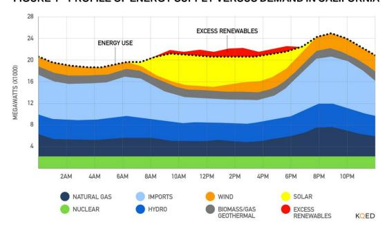
FIGURE 1 - PROFILE OF ENERGY SUPPLY VERSUS DEMAND IN CALIFORNIA
