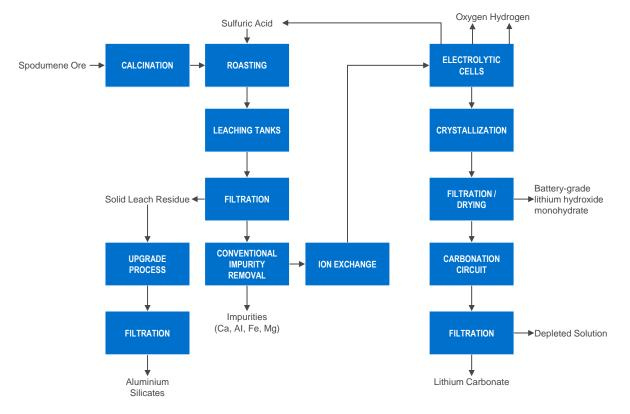
Figure 4: Illustrative Block Flow Diagram of Nemaska Lithium's Technology
